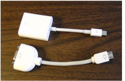
a different adapter. Immediately below: (upper: newer); (lower:older). The end that connects to BTI's VGA is shown at lower left corner (newer on left and older on right). The end that connects to the Mac is shown at lower-right (older on left and newer on right).
