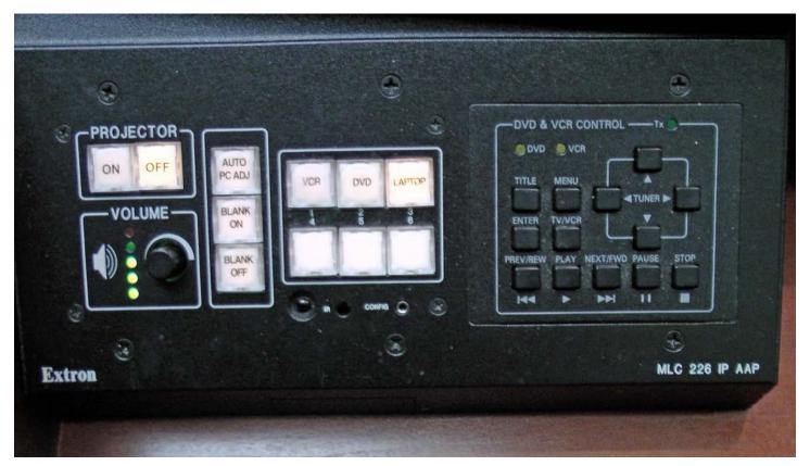
The projector off/on button is at the top-left of the control console. Pressing the ON button turns the projector on. The "ON" button will flash until the projector has warmed up.
