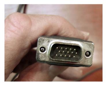
The video and audio connectors at the podium are shown above. THE PRESENTER is responsible for providing the proper connector between his/her laptop and this 15-pin VGA video cable. The newest (thinnest) Macintosh laptops use a "Mini DisplayPort to VGA Adapter;" older Macs use
